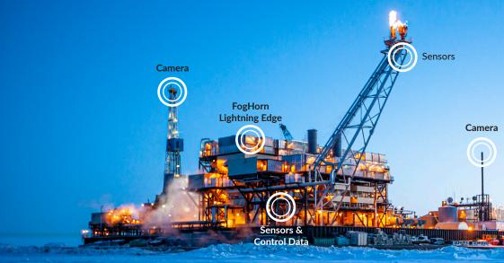
In this example, sensor fusion technology is employed to monitor flare stacks in oil refining. Live video streams of flares are combined with audio and vibration data and analyzed with deep learning models at the edge.
